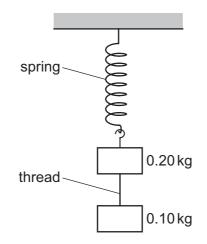
Immediately after the thread is cut, what is the upward acceleration of the 0.20 kg mass?
