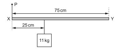
Which vertically upward force acting on end Y of the rod would hold the rod horizontally in equilibrium?
